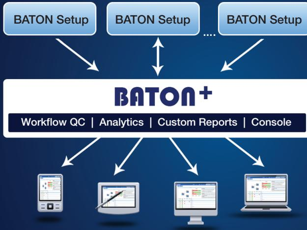
Interra Systems' BATON+ is an add-on tool in the BATON suite that works across multiple BATON installations and provides new functionalities over the core file-based QC functions provided by BATON: Workflow QC, Data Analytics, Custom Reports, and Management Console.
